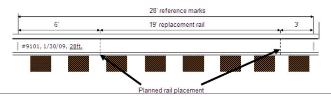
In the example below, when the rail was cut, the rail gapped open 1  $\frac{1}{2}$ ". The replacement rail was installed and after the joint bars were applied the distance between the reference marks is now 28 feet 1  $\frac{1}{2}$  inches. Document the 1  $\frac{1}{2}$ " added as a (+) measurement. The 1  $\frac{1}{2}$ " of rail added must be removed when the permanent repair is made.
